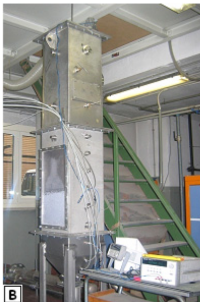
Fig. 7B. 0.35 m side square-based AISI 316 SS unit with tempered glass frontal window.
